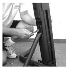
Then go back and **TIGHTEN FULLY** the <u>TOP</u> lock nut on the tubular brace.
