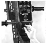
may use the resistance to control their climbing speed—by slowing the step speed down. The hydraulic control knob is located at the bottom of the control console.
