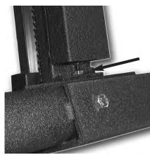
The hex head nut is tightened down against a flat bar, so you'll need a 7/16" open end wrench to loosen it. Loosen the nut away from the flat bar about 2 turns. With the same 7/16" wrench tighten the hex bolt deeper into the flat bar
