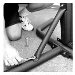
Next, tighten the  $\underline{\mathsf{BOTTOM}}$  lock nut on the back brace to complete post assembly.
