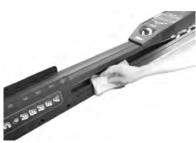
First wipe any excess oil, lint, dirt, etc. from all internal accessible surfaces of the rectangular tubing. Move the bars up and down to allow access to clean the two foot
