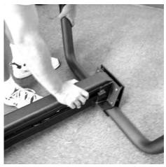
Attach the front curved tubular floor brace to the post. Using four hex head bolts, 3/8" x 5/8" long bolts, screw down until firmly tight.
