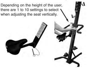
This comfortable seat is adjustable vertically with the pin and horizontally with a knob located under the seat. The vertical seat adjustment is for differences in leg lengths while the horizontal adjustment accounts for differences in arm lengths.
