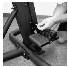
Attach foot pedals with "L" shape bracket pointing up, using (2) 3/8" x 11/4" long hex head bolts.
