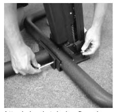
Attach back tubular floor brace to post with two hex head bolts, 3/8"x 33/4" long. (2) 3/8" lock nuts. **DO NOT TIGHTEN FULLY AT THIS TIME.**
